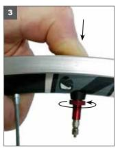
3. Firmly press the base of the valve into the rim with your thumb and finger-tighten the knurled nut.
