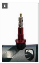
Before riding make sure the valve is closed and check that the silver valve core and red knurled nut are finger-tight.
