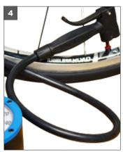
4. When using a pump be careful not to bend the valve with the pump head. When removing pump head, pull straight off and avoid twisting or sideways movement.
