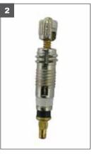
2. Once the silver presta valve core is removed, coat it with Tri-Flow® or a similar lube inside and out. Lube prevents the valve from clogging with sealant.
