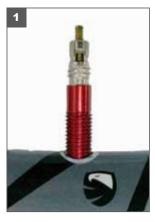
1. Insert red valve stem with the two (2) rubber O-rings into the tire well.
