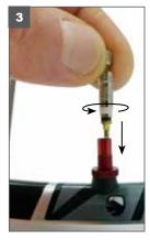
3. Reinstall the valve core, finger-tighten only. Do not use a wrench or pliers to avoid stripping the aluminum threads in the valve.
