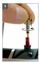
1. With the valve installed, unthread and remove the valve core using pliers or a valve core removal tool.
