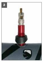
2. Use the plastic contoured spacer to protect the rim from the knurled nut.
