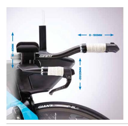
In addition to refined frame geometry, Giant engineers improved the range of adjustability while simplifying the cockpit configuration to fit a wider range of riders more easily.
