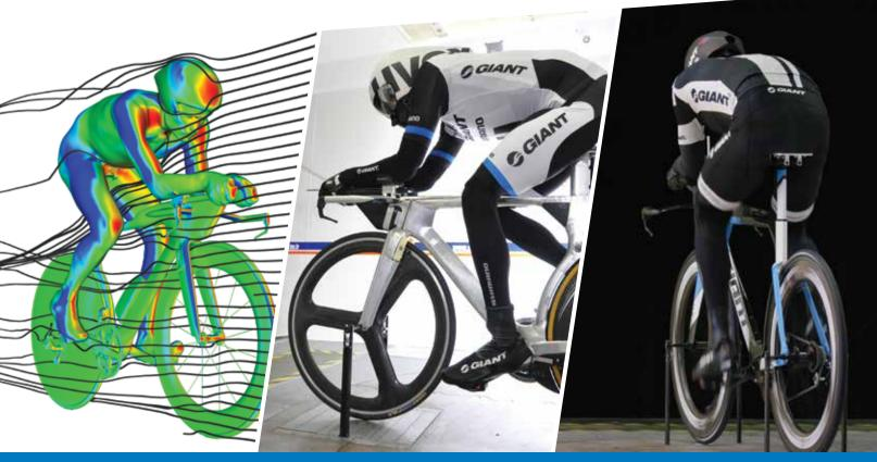
(From left to right) The development process begins with extensive analysis using Computational Fluid Dynamics (CFD). Dynamic testing in the wind tunnel using an aluminum prototype frame and the Grischa mannequin allows Giant engineers to test frame designs in real-world conditions. Production sample wind tunnel testing verifies Trinity's performance before commercial release.
