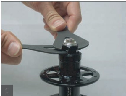
1 Using two 19mm cone wrenches, remove lock nut and adjusting nut.
