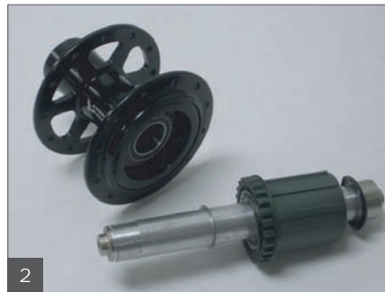
2 Separate cassette body and axle from the hub shell by grabbing the body and pulling out from the drive side.
